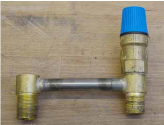
Dismantled bypass unit.
